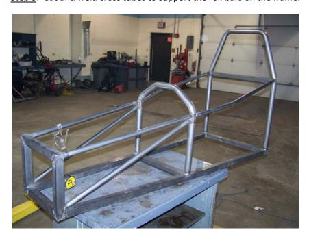
Step 4: Weld "halo" bar to frame and connect crose bars to reinforce the halo bar.
