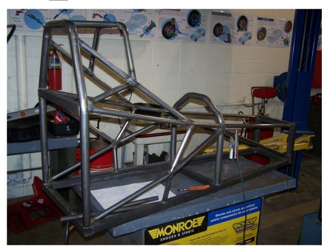
With the frame 100% fabricated and welded, our next step will be to mount the front axle and figure out a mounting system for the engine and rear axle. This year we are continuing to use the Briggs and Stratton horizontal shaft motor connected to a live axle. We hope to have the car on the tires by the end of Feburary.
