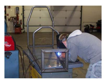
Step 3: Cut and weld cross tubes to support the roll bars on the frame.
